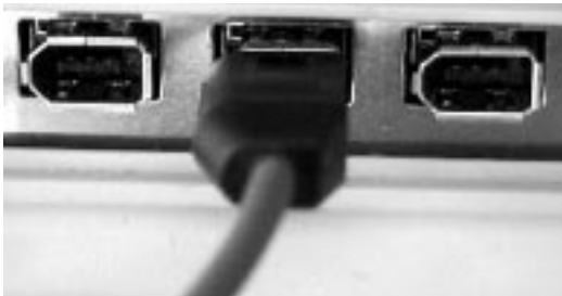
Connecting the cable to the Digital Origin 1394 FireWire card
